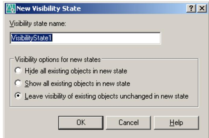
5. Make the electric coils on the range top invisible in the current (Gas) visibility state.
