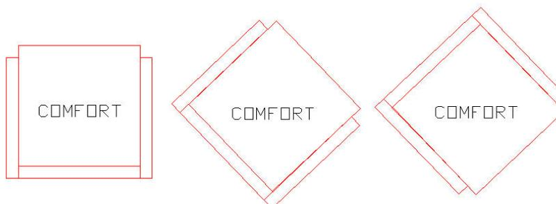
The above example of a chair block with an attribute value for the type of chair does NOT rotate when the chair is rotated. This gives you the ability to have attribute text stay at the zero-degree angle or horizontal, making it easier to read. There are two schools of thought on this, depending on how you typically manipulate the block.
