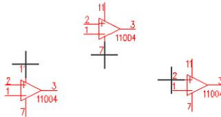
Block definitions can contain multiple representations of a particular symbol. Upon insertion, you can choose which representation to use. For example, a single block definition could store multiple representations of a bed, faucet, door or valve.
