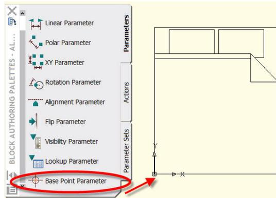
**Tip Revealed:** To correct this problem, simply open the block inside the Block Editor and attach a base point parameter from the authoring palette. Save the block. Any existing blocks of that name or future instances of that block will have the correct insertion point.
