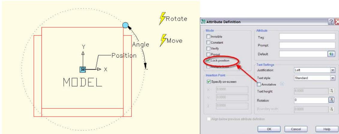
**Tip Revealed:** The common mistake here is NOT to lock the position of the attribute. Locking the position actually locks the orientation, which stops the attribute text from spinning or rotating when you rotate the block. Note that in the attdef dialog box above there is an option for locking the position of the attribute. If you forget to lock the position, you can change that property using the property palette inside the Block Editor. That’s wicked cool!
