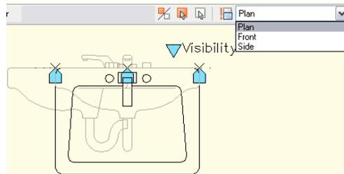
**Tip Revealed:** Although you can create individual parameters for each action, that would require you to grip edit three different times (one for each action). Instead, create one parameter and let it drive all three actions. In this example, you know you need a parameter that supports the Move, Stretch and Scale actions.
