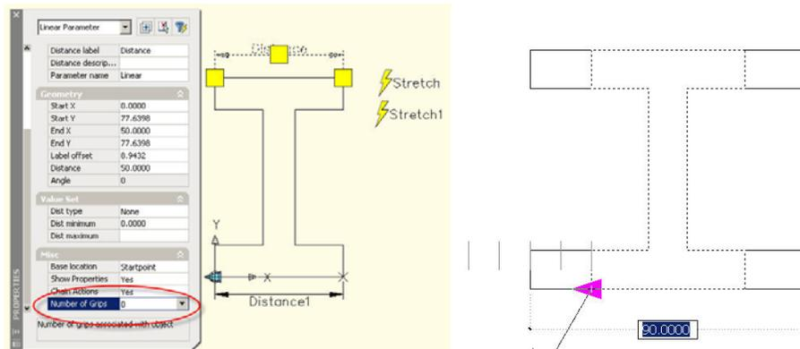
This technique is commonly used when you have two or more actions associated with the same parameter or multiple parameters chained together. This gives you better control by only displaying the parameters you need to edit when you insert the block.
