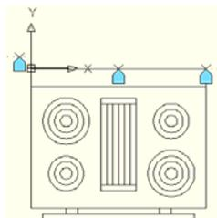
The base point parameter defines a base point for the Dynamic Block reference relative to the geometry in the block, overriding the default origin point of the block. Like the alignment parameter, the base point parameter does not require any actions, but can belong to an action's selection set. The base point parameter displays in the Block Editor as a circle with crosshairs.
