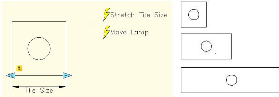
In the reflective ceiling tile example, we have one parameter and two actions. By editing the location of one of the linear parameter controls, it does a “Stretch” action on the size of the tile while doing a “Move” action on the circle (lamp) to maintain its location in the center of the tile.
