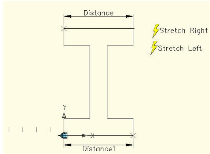
In this modified version of the I-beam, chaining allows me to stretch both sides at the same time using just one parameter control grip to activate the action of both sides stretching.
