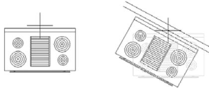
As you insert a Dynamic Block, you can cycle between key insertion points to find the one that makes the most sense for your current situation. The ability to cycle through insertion points can eliminate the need for you to move the block after it is inserted.
