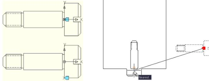
For some blocks, you might find it useful to include multiple insertion points. For example, when inserting a stove block, you might want to insert it using the left corner, the right corner, or the center, depending on the other geometry in the drawing. You can define your blocks with multiple alignment parameters and then use the CTRL key to cycle between the alignment grips upon insertion.
